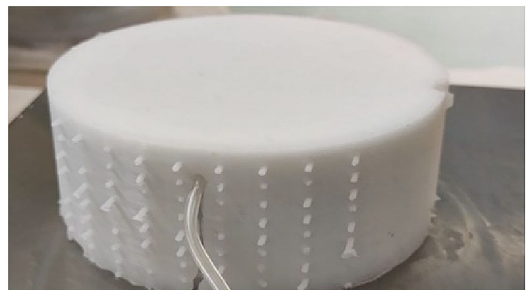
Fig. 1 Silicone phantom with a tube inclusion at the depth of 5 mm. The phantom is a cylindrical phantom of 120 mm in diameter and 45 mm in thickness with a cylindrical inclusion of 3 mm in diameter and 120 mm in length at a depth of 5 mm
