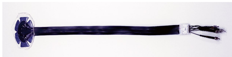
Fig. 1 Sensor used in measurements. Four SMA connectors are connectors to LED light sources and two are connected to the APDs
